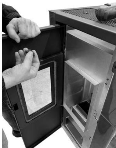
Fig. 19 - Remover a dobradiça
